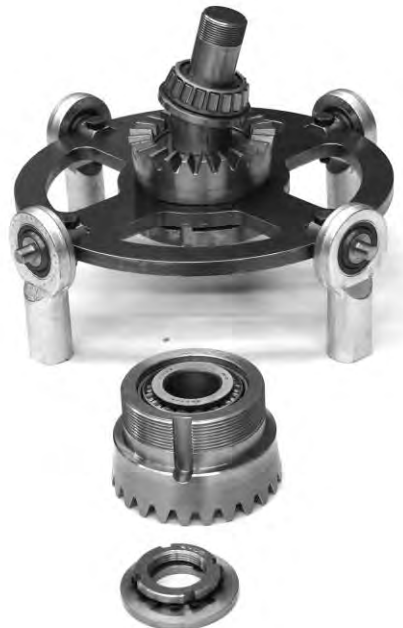
Figure 5: Swing plate with rod ends, crankshaft, bearings and gear wheels
