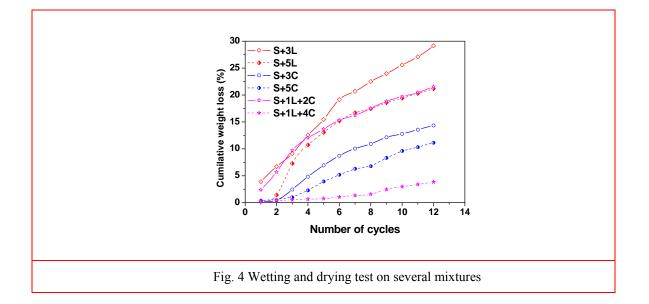
It can be concluded that the addition of lime or a small amount of cement slightly influenced durability resistance, while an additional amount of cement will lead to a significant decrease in weight loss and therefore, a good sustainable resistance of pavement layers prepared within the combined treatment of silty soil.
